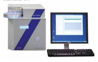
The QFID-100HR measures automatically samples of all kinds. He includes both, a headspace- sampler and a gas chromatograph. Fast, reliable and with a very high precision the headspace-samples will be analyzed. The instrument can separate 18 most important solvents (the analyses of different solvents is possible). A complete analyse of a 20ml HSS-vial needs approx. 8 minutes. The result will be printed out in mg/m², for example.
